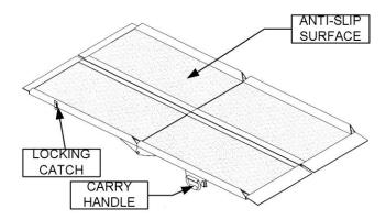
The SMART RAMPs can be used either as a portable or fixed access ramp. The ramps are suitable for a single PMV with user. PMVs (Personal Mobility Vehicle) are wheelchairs, powered wheelchairs and scooters. The ramps can be used to obtain access to motor vehicles, buildings, etc.
